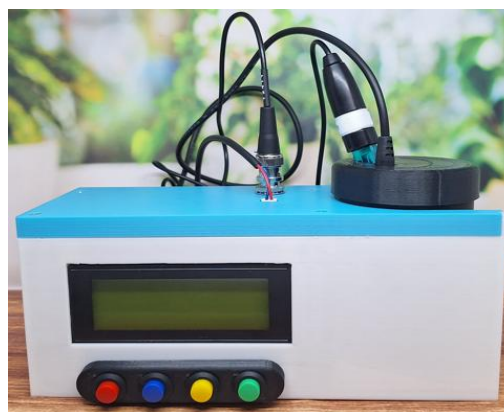
FIGURE 6. The front panel of the device is equipped with a liquid crystal display (LCD) for presenting measurement results. The red, blue, and yellow push buttons are designated for solution calibration procedures, while the green push button is used to initiate the sample testing process
