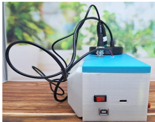
FIGURE 6. The side view of the device shows the main hardware interfaces, including the power on/off switch, the
