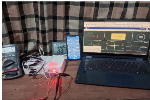
FIGURE 8. Simulating Diagnostic Signals Via DB25 Port
