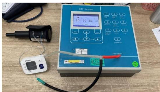
Figure 5 Installation of the BPM and NIBP Simulator
