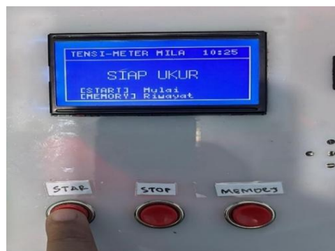
Figure 5 Initial Display of LCD Screen on blood pressure measurement system design equipped with audio information and measurement memory
