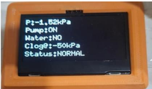
FIGURE 5. The device starting up display, the “maximum pressure” as well as if the device has an error or not currently.
